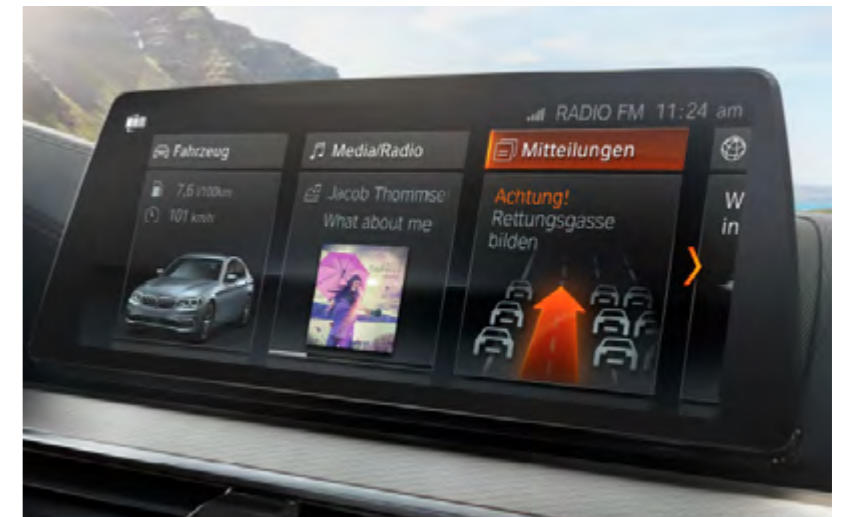
Warning, emergency corridor: authorities can send drivers warning messages to the screens in vehicles with ConnectedDrive.
