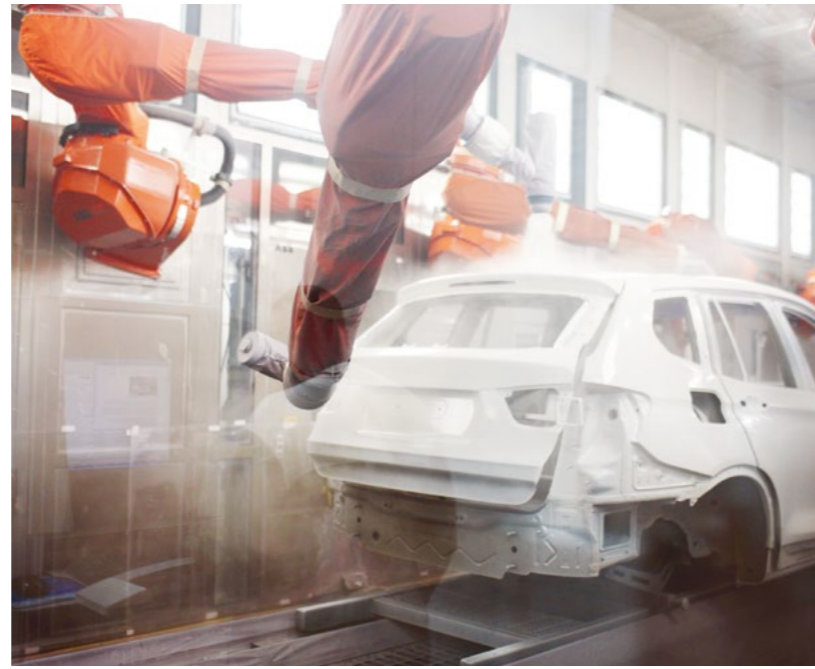
REDUCING WATER CONSUMPTION — Modern dry scrubbing method in the paint shop at the BMW plant in Spartanburg.
